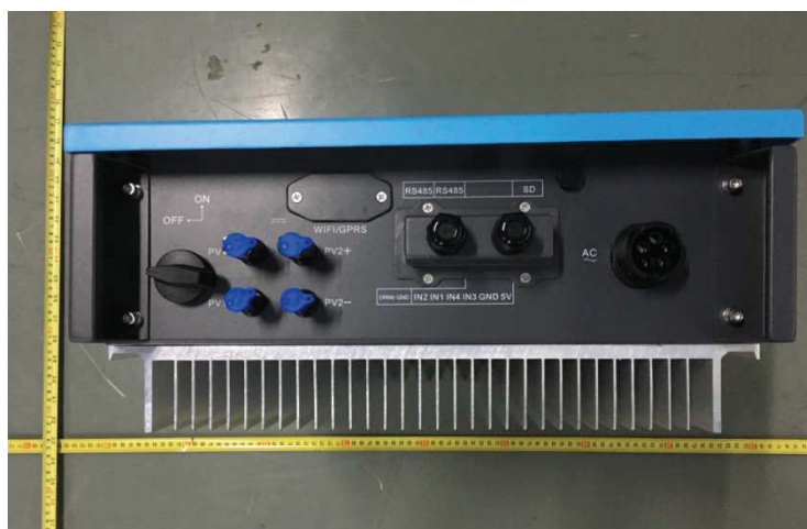
Figure 2. View of terminals
